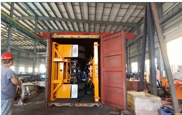
Two units flatbed trailers load by 40FT High container
