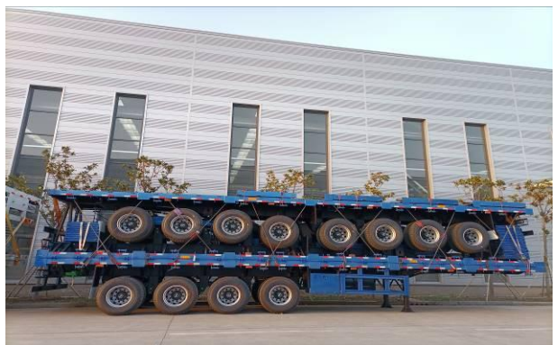
Three units flatbed trailers fold and load by bulk ship
