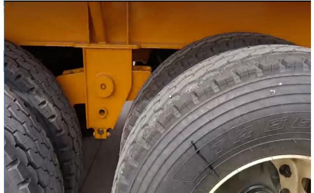
Heavy duty design suspension hanger Main beam thickness 14 /8 /16mm, Durable chassis
